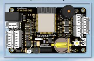
Your key to extended two-way communication. This powerful pair, featuring a Master and Slave device, excels at effortlessly extending the distance between your reader and controller by up to **100m**. It seamlessly converts Wiegand protocol, MicroID 485, pushbutton, and relay signals to wireless, simplifying your access control setup. With **encrypted** communication, the **Smart**Converter propels your system to new distances.
