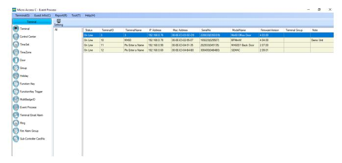
2 • Then click "Setting" button to call an Event Process configuration window as shown. There are "Event Triggered Level", "Event duration", "Trigger level", "Alarm" and "IP Camera" information should be configured.
